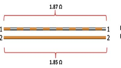
Resistance = 3.7 Ω Resistance Unbalance = 0.02 Ω
