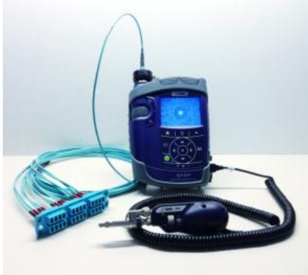
Patch Cord (“Male”) Inspection
