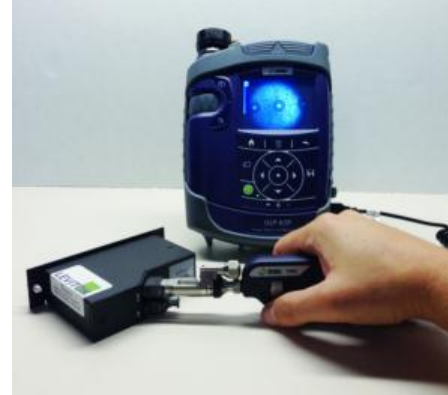
Bulkhead (“Female”) Inspection
