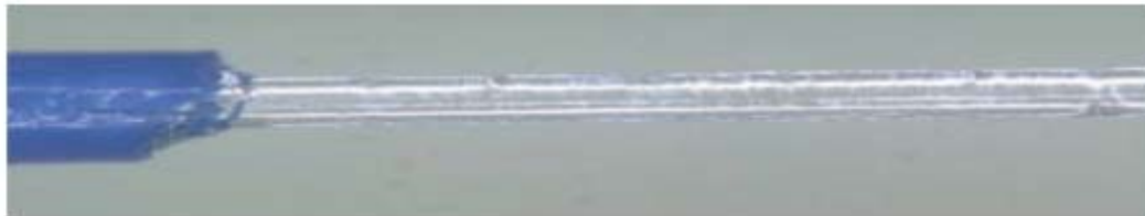
(b) Scratching caused by coating debris
