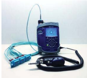
Patch Cord ("Male") Inspection
