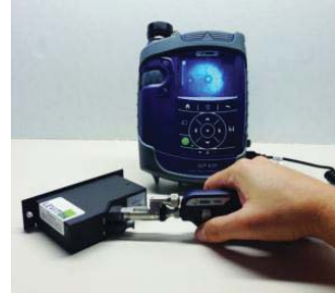
Bulkhead ("Female") Inspection
